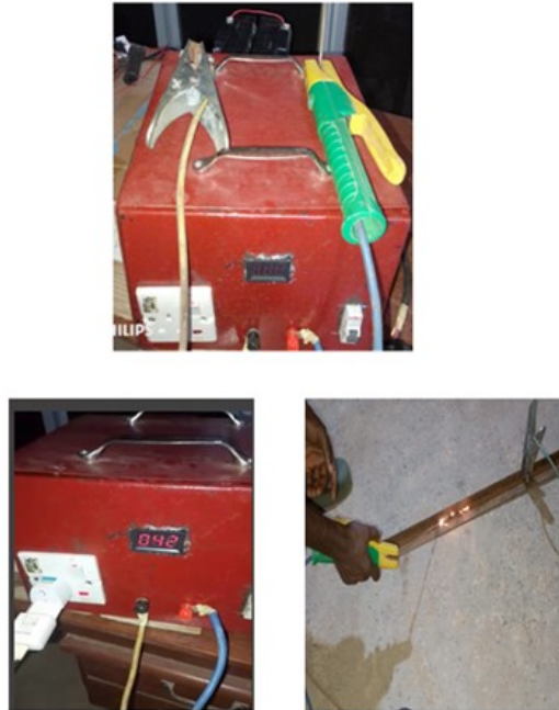
Figure 1: Compact prototype design of the solar-hybrid welding machine (excluding solar panels).
