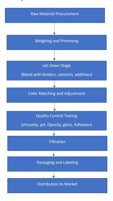
Figure 2.1: Proposed Process for Commercial Production of Paint
