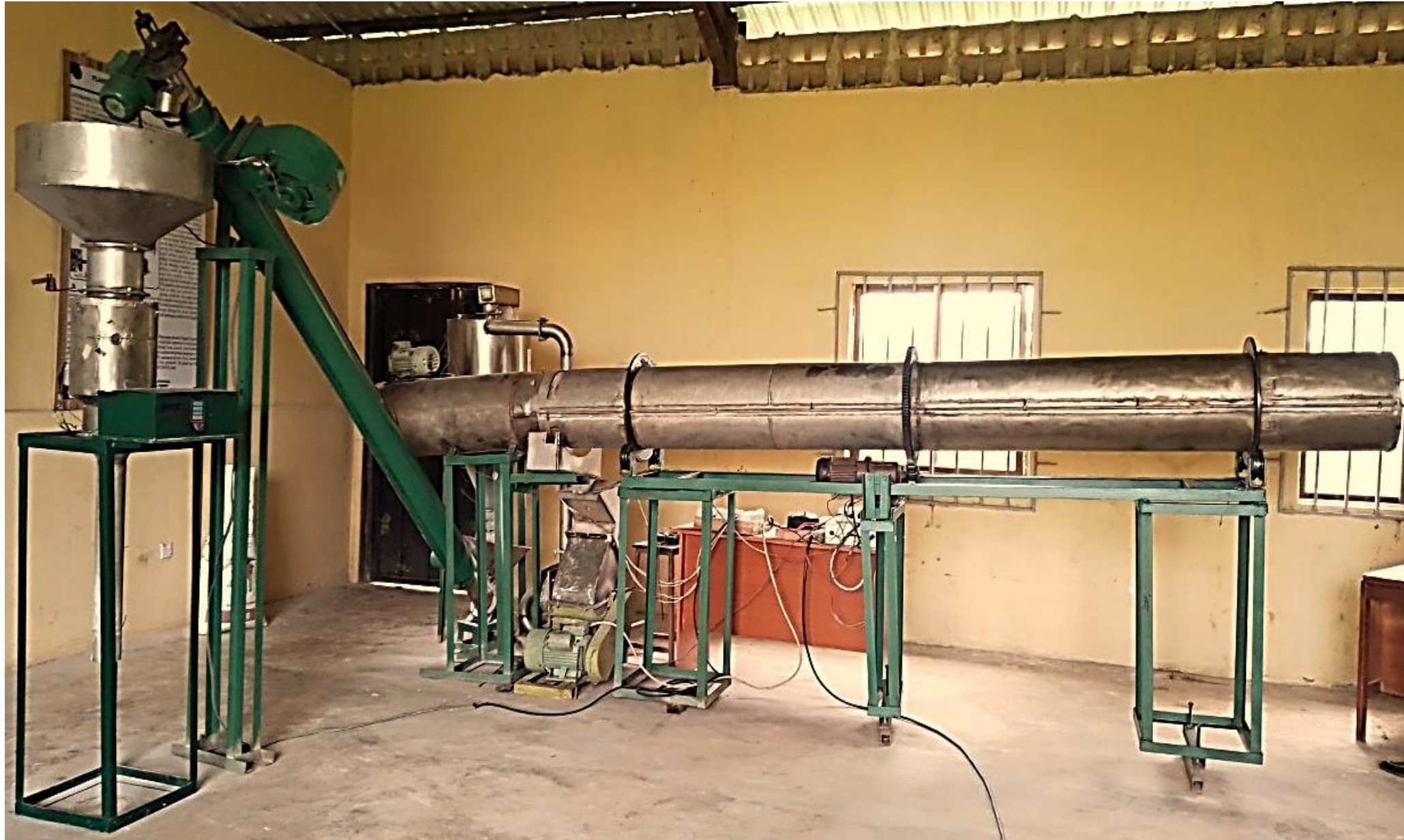
Plate 1: Assembly of the Fabricated Sections of the Plantain Processing Plant
