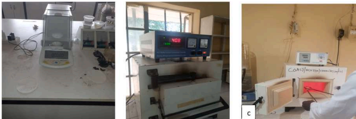
Fig. 3. Glass fabrication process (a) Digital Weighing Balance (b) Preheating Muffle furnace (c) Melting Muffle furnace.
