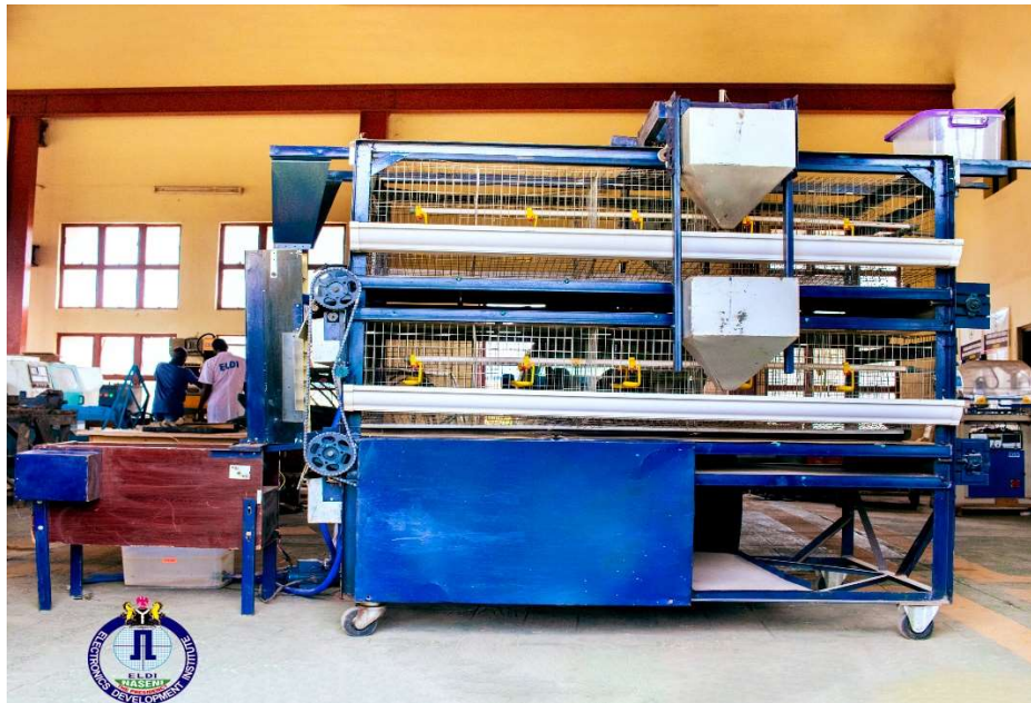
Figure 2: Automated Poultry management system for Battery cage system showing the side view.
