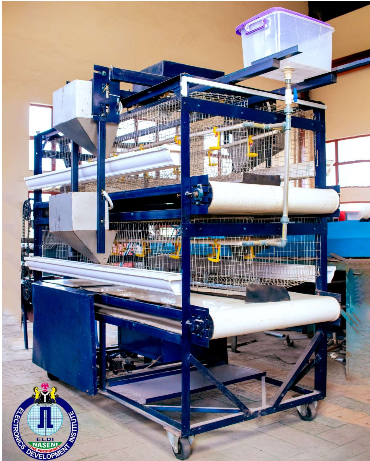
Figure1: Automated Poultry Management System for Battery cage Showing the back view
