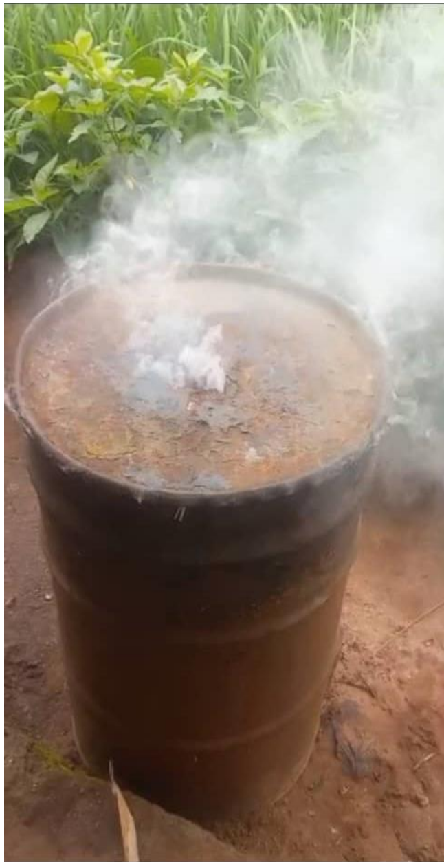
4. Activated charcoal feed additive produced from biomass waste using pyrolysis
