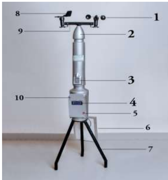
Figure 4: Front view of the IoT mobile solar powered weather station.
