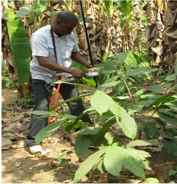
Plate 3: Gas exchange determination with IRGA machine on the budded plant by Ayegboyin
