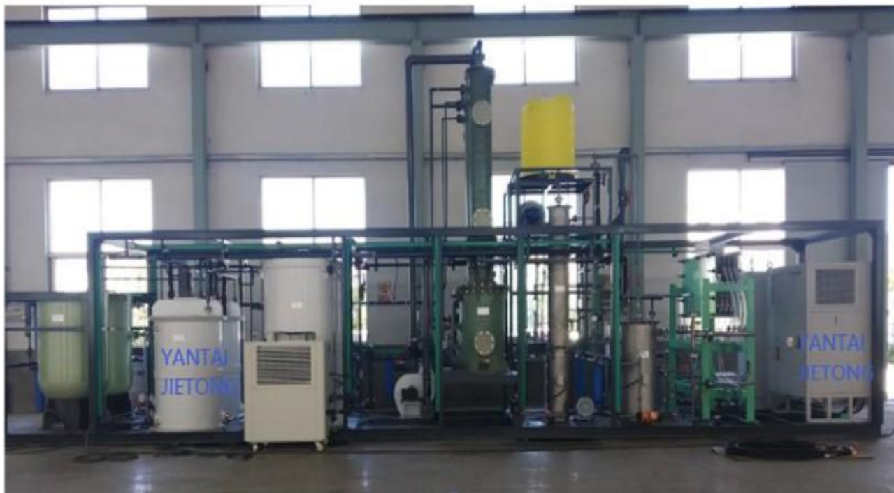
Plate 1: The Turnkey Plant expected from China for the Production of Sodium Hypochloride, Sodium Hydroxide, Chlorine Gas etc.
