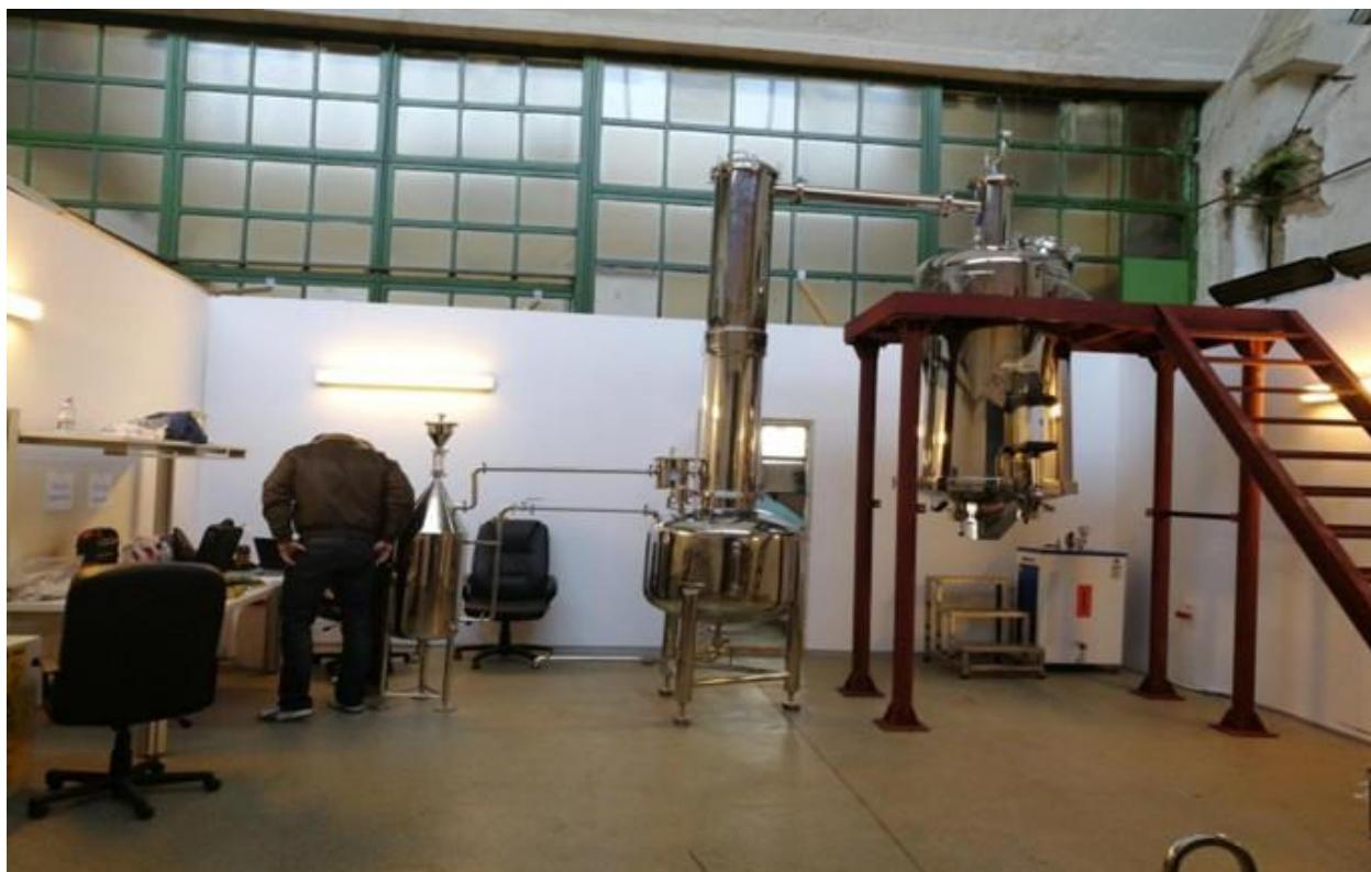
Fig. 1. Picture of the proposed Industrial-scale 1000 liter capacity steam distillation equipment for the essential oil extraction.
