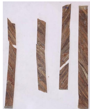
Figure 9. Fractures specimens of untreated treated 10% SSD fibre at 45-degree Orientation
