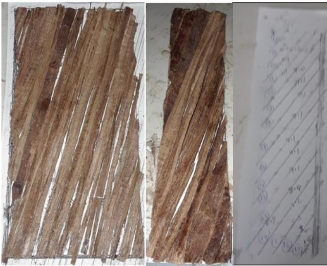
Figure 1. (a) Fibre placed on the paper at angular orientation for tensile and flexural composite production (b) Fibre placed on the paper for compression test specimen (c) Paper with drawn angular orientation for fibre placement
