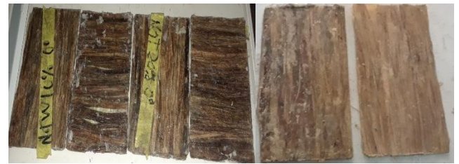
Figure 3. SSD fibre-epoxy composite produced at 0-degree and 90-degree orientation
