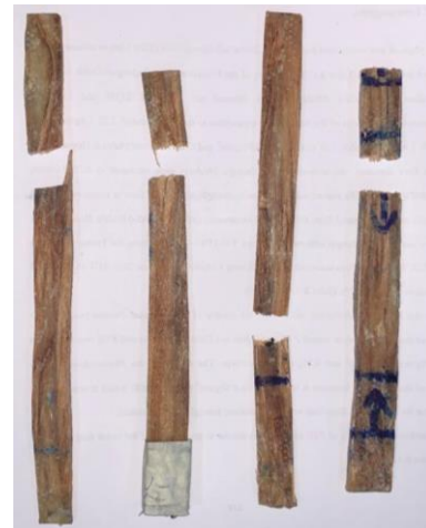
Figure 8. Fractures specimens of Hot Alkaline treated 5% SSD fibre at 0-degree Orientation
