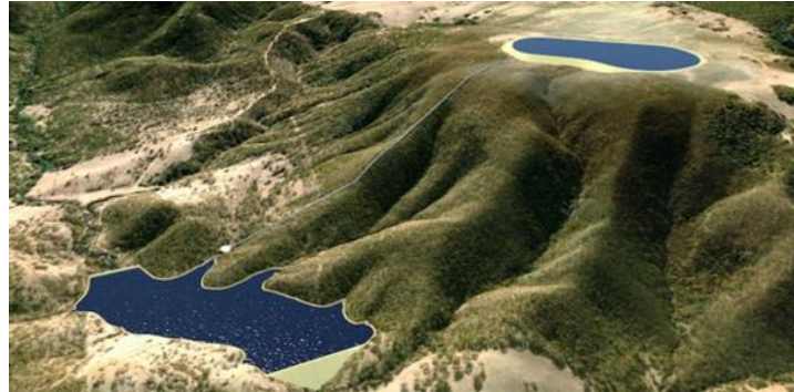
Figure 2: A lower and upper reservoir of a pump hydro storage ( https://www.atco.com/en-au/about-us/stories/atco-pumped-hydro-storage-nsw.html )
