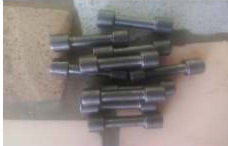
Figure 11: Tensile test samples
