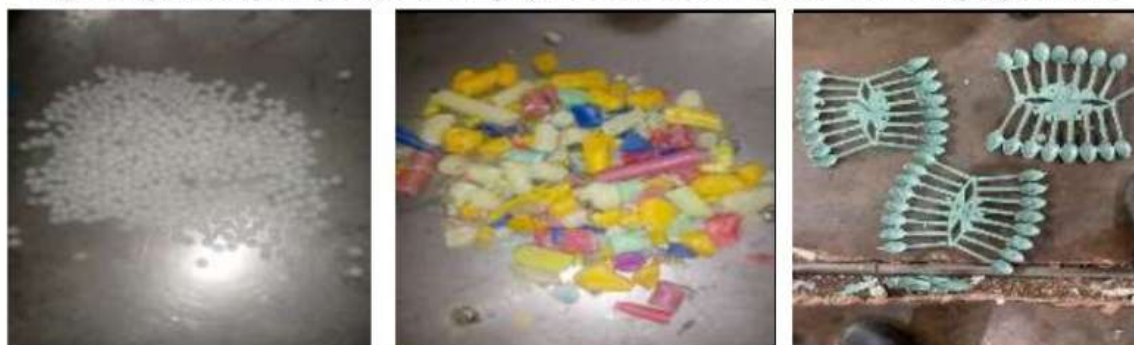
Fig 6: Disposable spoon produced from blend with PP and polymer crush
