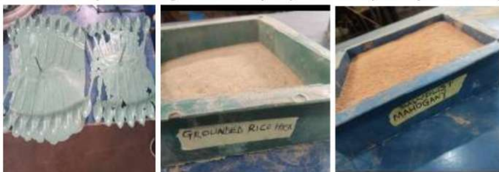
Fig 5: Disposable spoon produced from polymer blend with Rice husk and mahogany sawdust
