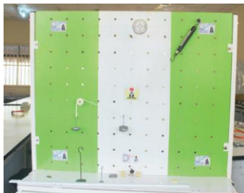
Fig.14: Triangle of Forces Principles Experimental Setup
