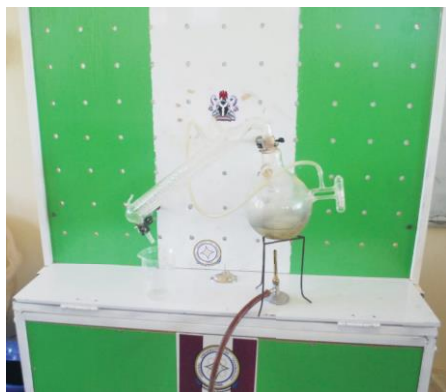
Fig. 18: Experimental Setup for Simple Distillation on the Mobile Laboratory
