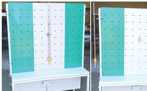
Fig. 12: Experimental Setup for Compound Pendulum a & b
