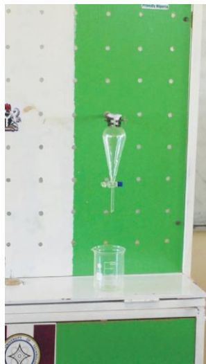
Fig. 17: Experimental Setup for Separating funnel on the Mobile Laboratory
