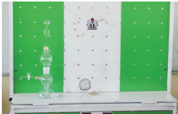
Fig. 22: Experimental Setup for Laboratory Preparation of Gases on the Mobile Laboratory
