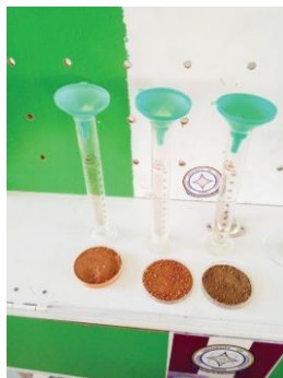
Fig. 23: Computing the Water holding Capacity of Different Types of Soil. (Fig. 20)
