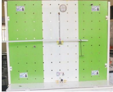
Fig 8 : Moment Principle with Meter Rule
