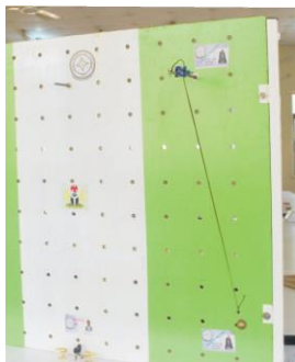
Fig.11: Experimental Setup for Simple Pendulum
